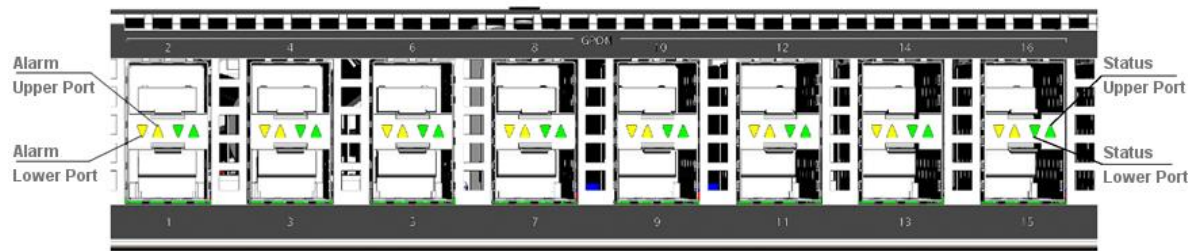
Figure 8 - GPON Ports and LEDs
